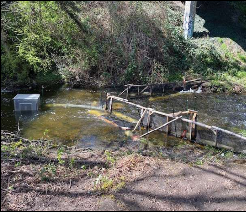
Figure 2: Smolt Trap installed by PSS
